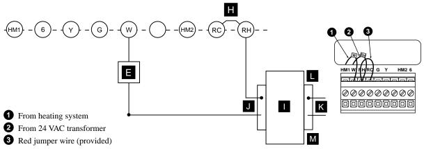
For humidifier wiring see pages 14-15. See page 9 for letter identification. NOTE: Ensure that RED RH/RC jumper wire (provided with thermostat) is connected between thermostat's RH and RC terminals for proper operation with this system.
